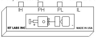
Connections to the measuring instrument are made through cables with BNC connectors which mate directly with the RLC Meter. The cables are coded to ensure proper connections.
